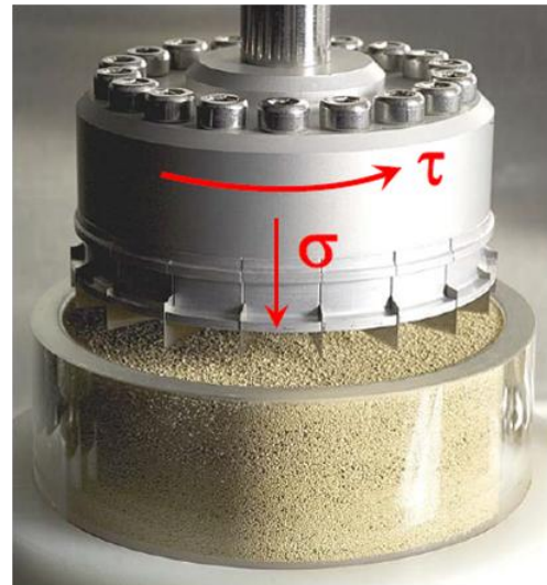
Fig 2: Shear cell configuration
